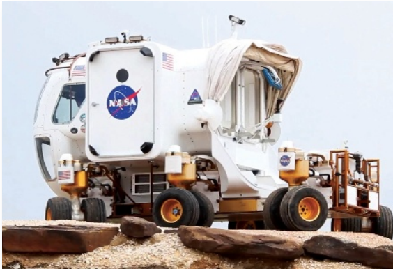
This rover includes about 70 FDM parts, including housings, vents and fixtures.
